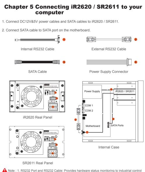
Note : 1. RS232 Port and RS232 Cable: Provides hardware status monitoring to industrial control system or IPC via RS232. If more information required, please contact at supporting@raidon.com.tw
